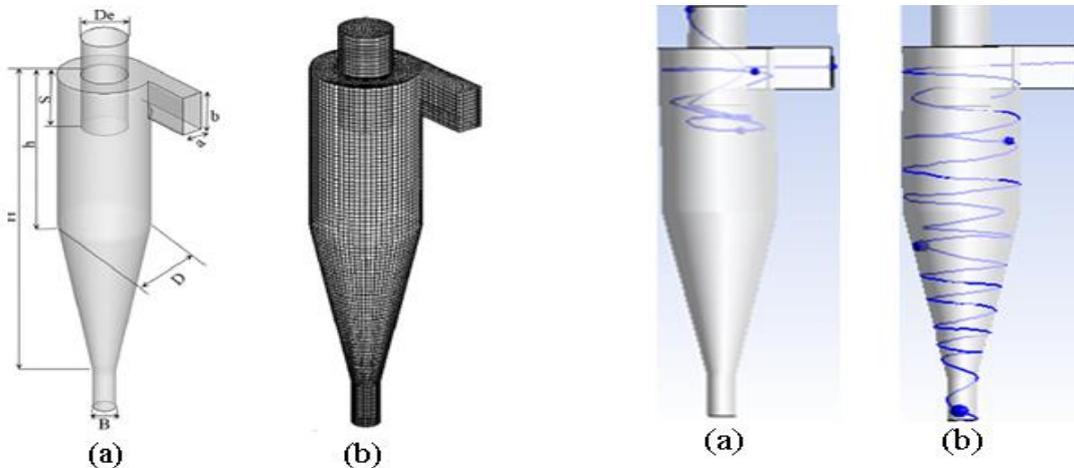
**Figure 1. Schematic (a) and grid representation (b) of the simulation cyclone**
