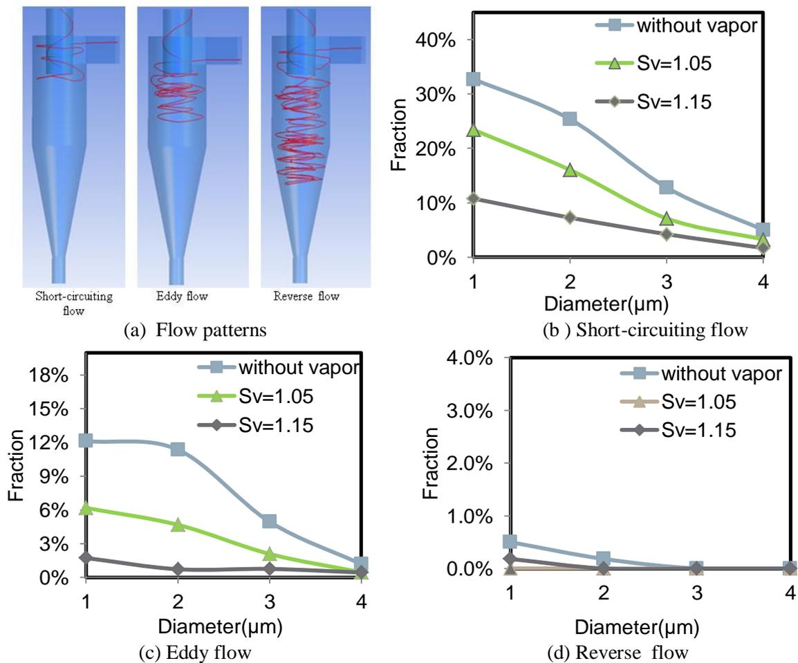
**Fig 5. Schematic of three flow patterns and the effect of saturation ratio on the fraction distribution of flow patterns**
