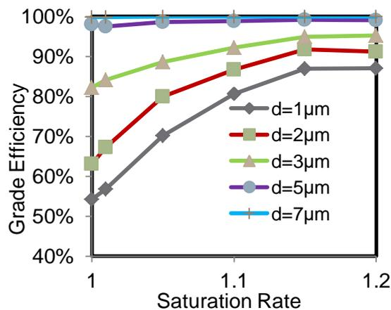
Fig 3. Collection efficiency as a function of saturation ratio for different sized particles
