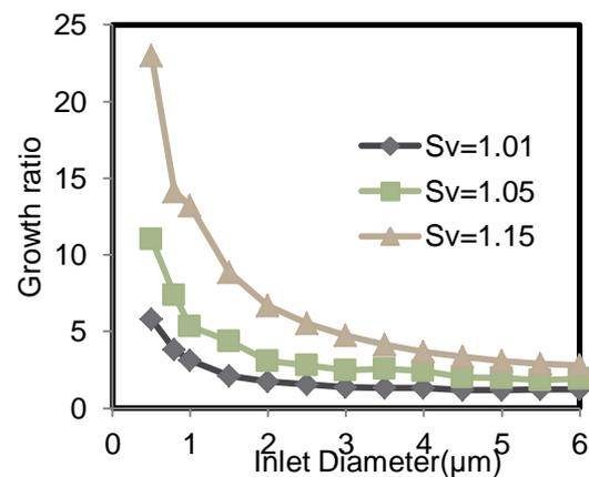
Fig 4. The effect of saturation ratio on the growth of particles of different sizes
