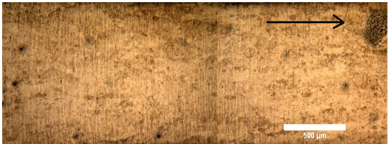
Figure 4 Optical microscopy of lateral view of SLMed Ti64.
